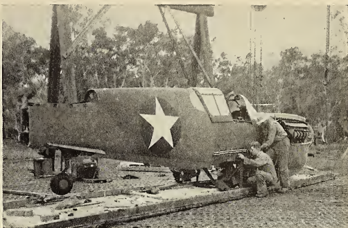
Hydraulic equipment might be better, but these mechs still do a good job of lifting this pursuit ship with an improvised hoist.
